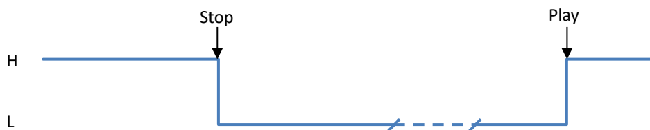
Figure 19 – Usage of the AUDIO_STATUS pin
