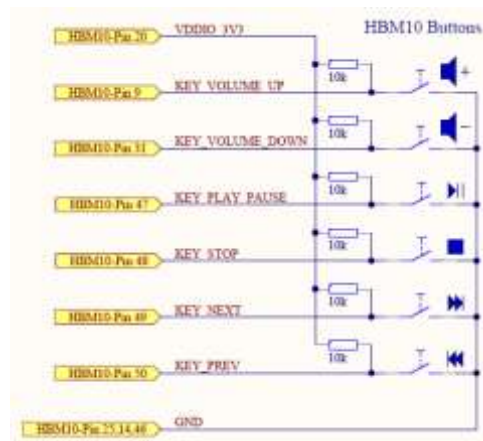
Figure 15 – Recommended usage of the Audio Pins
